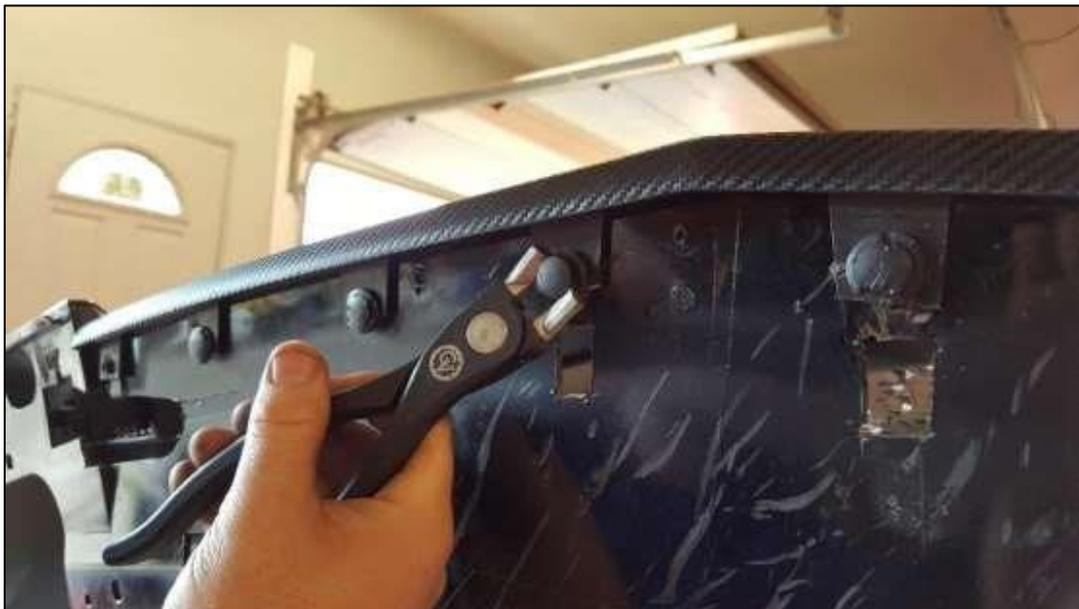
6. Once the 2- 7mm bolts and 6 push pins are removed, pull the center trim piece out. Drill/enlarge the hole in each tab to 3/8". The supplied **Stainless Steel 1/4" x 1 1/2"** mounting bolts for the splitter will now pass thru these enlarged holes. They might need additional clearance once the splitter is bolted up.
